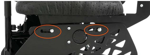
Then set the desired height by placing 4 screws in the holes at the same level. Finally, all screws must be tightened firmly.
